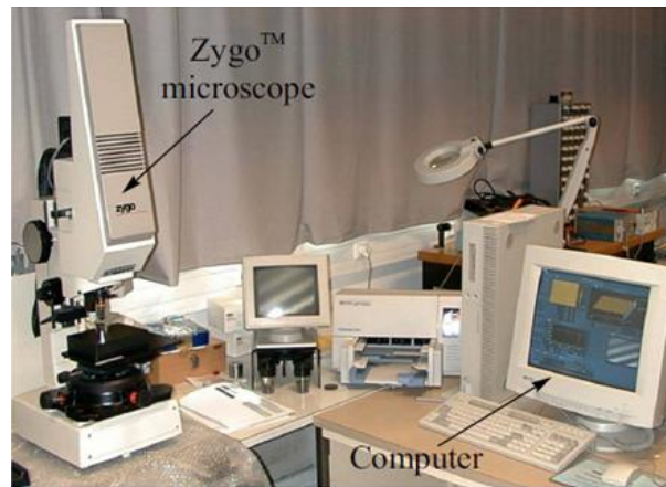
Fig III-3: Real view of ZYGO™ 200 interferometer microscope
