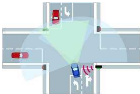
Figure 1 : The figure illustrates the intersection management problem: a communicating system between the vehicle and the traffic light as well as prevention of collision with other vehicles are illustrated.
