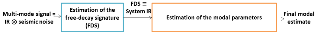
Figure 2.3: The general overview of the two steps of the output-only modal analysis.
