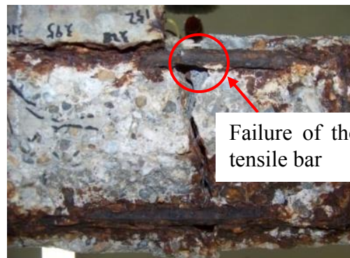
Figure 5-3 Experimental test on the corroded beam B2C13
