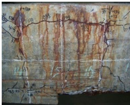
Figure 5-3 Experimental test on the corroded beam B2C13
