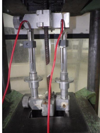
Figure 4-2 Uniaxial tension tests on the bars
