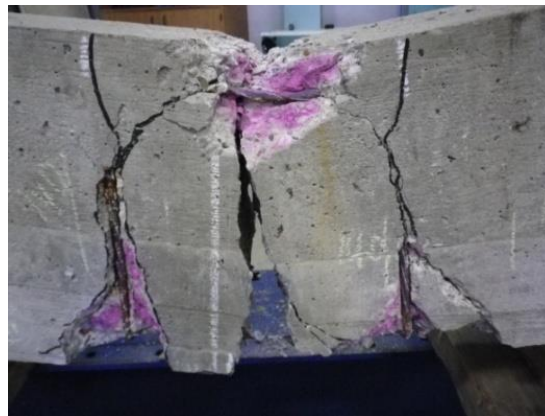
(b) Failure of the non-corroded beam B2T2 due to concrete crushing
