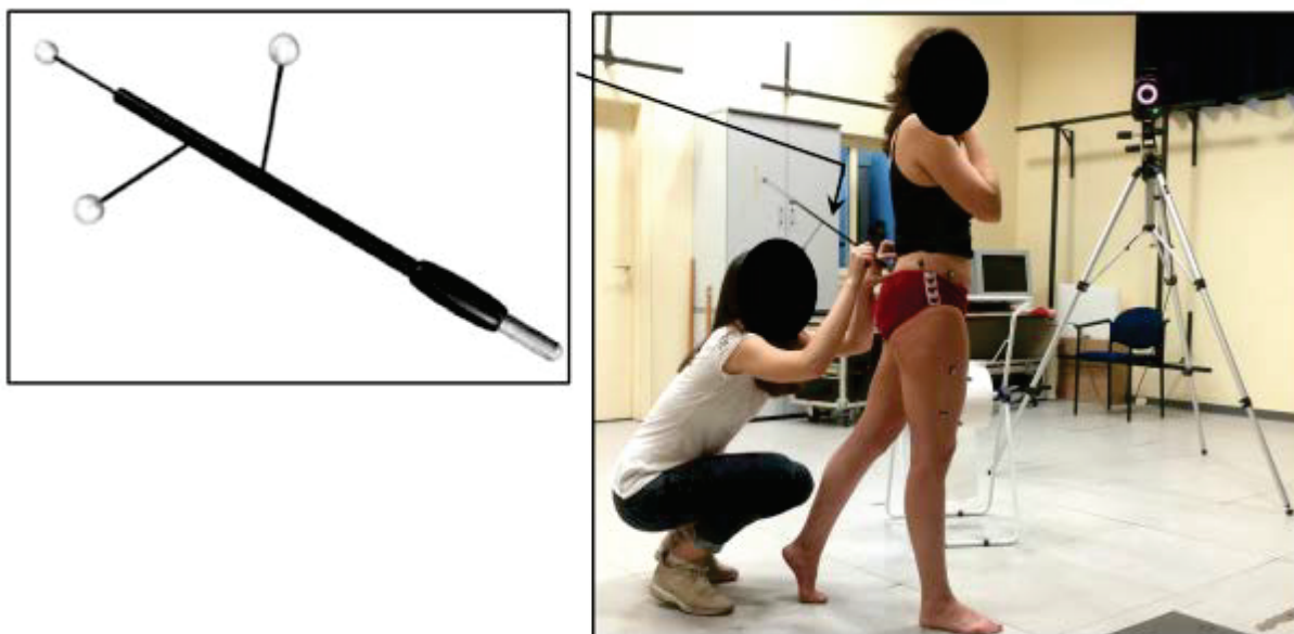
Figure A2.10 – Identification procedure of the position of a pelvic AL during the toe-off posture of one subject using the wand equipped with three markers and a rolling tip.
