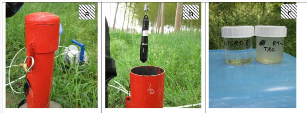
Figure 21. Installed piezometers in Monbéqui study site. ‘a’ shows the piezometer, ‘b’ shows the water level sensor installed in the piezometers, ‘c’ shows sampled groundwater.
