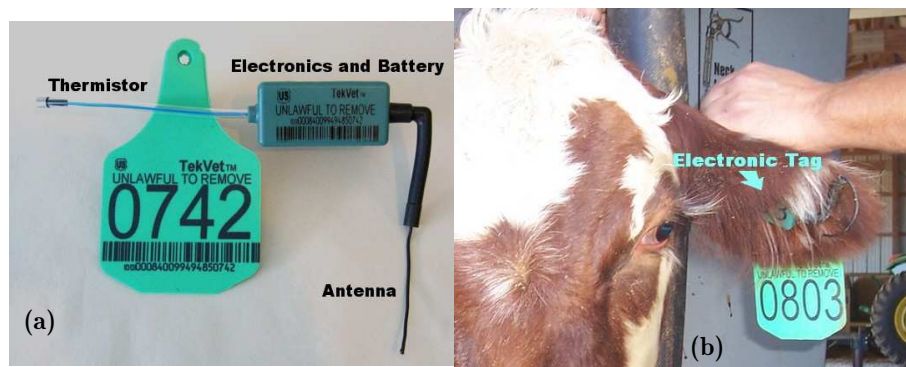
Figure 6.3: An active tracking device to track livestock, developed and industrialized by Tekvet and IBM [357; 358].
