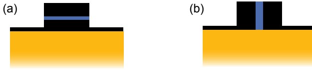
Fig. 4.5 Examples of cross-sections for a (a) horizontal and (b) vertical slot waveguide. The thin, unetched silicon layer is not needed for passive waveguides, but can be used to electrically contact the silicon block(s) in active devices.
