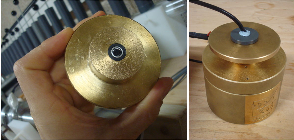
Figure C.1: Detail of the third microphone head and its attachment to the AIS for calibration.
