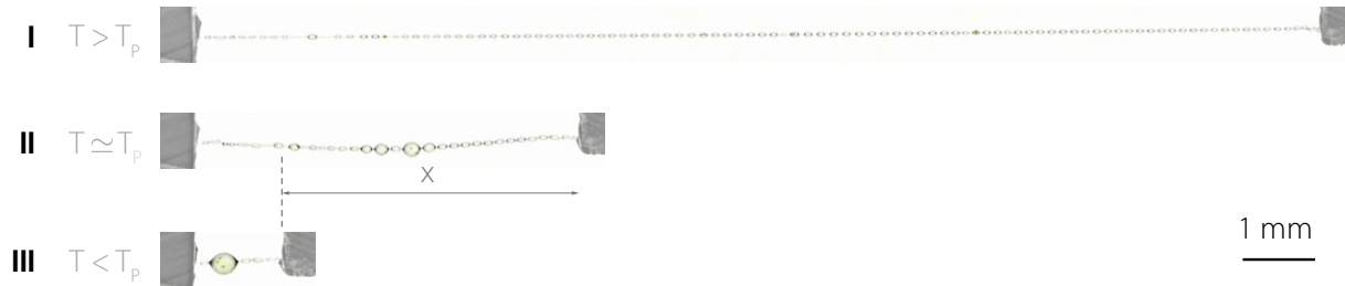
Figure 1. A liquid-like fibre. Whether stretched or relaxed, the typical capture silk thread of an araneid orb spider (here Nephila edulis ) remains taut. Force monitoring reveals a threshold tension T_P above which the fibre behaves like a spring (I). As the force is decreased a force plateau T \approx T_P is reached, along which the fibre adopts a wide range of lengths, just as soap films do (II). At lower forces, T < T_P , the fibre is totally contracted (III). See also Supplementary Videos for full cycle.
