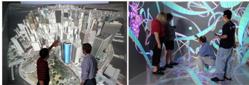
Figure 2-8: The six-channel CAVE system, the 10' x 10' environment features wireless tracking and communication devices and a three-dimensional audio system, IOWA State University [IOWA 2013]
