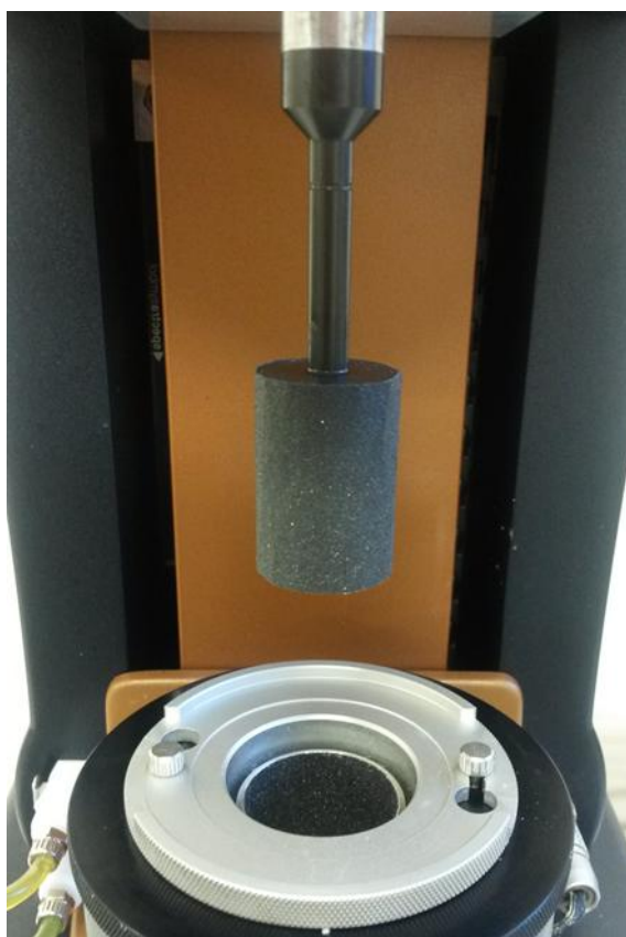
Figure C.2 The photograph of DHR-3 rheometer equipped with serrated (roughened) Couette geometry manufactured by gluing the sandpaper to the available Couette with smooth surfaces
