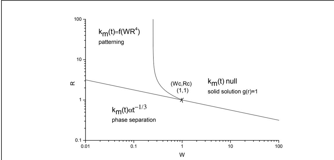
Figure 1: According to the reduced values of  $R$  and  $W$ , three distinct domains can be drawn. These domains are associated to a phase separation (low  $W$  values whatever  $R$  values are), a random solid solution ( $W$  is important and  $R$  above 1), and a steady state. This steady state is defined by a given value of  $k_m$  that only depends on  $W$  and  $R$ . As displayed on the graph, a critical point  $(W_c, R_c)$  equal to  $(1, 1)$  appears.
