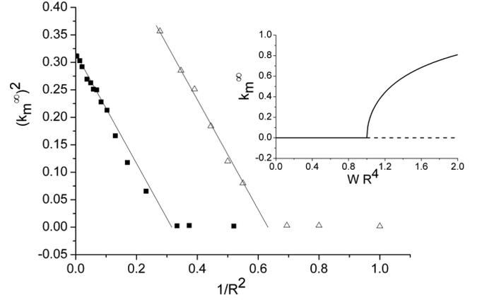
FIG. 2. Variation of  $(k_m^\infty)^2$  extracted from numerical simulations (black squares:  $W = 0.1$ , open triangles:  $W = 0.4$ ) for large times ( $t > 100\,000$ ) as a function of  $R^{-2}$ . The evolution of  $(k_m^\infty)^2$  exhibits a linear variation as expected (full lines), for  $WR^4 > 1$ . For  $WR^4 < 1$ ,  $(k_m^\infty)^2$  is null. The inset displays the evolution of  $k_m^\infty$  with  $WR^4$ .
