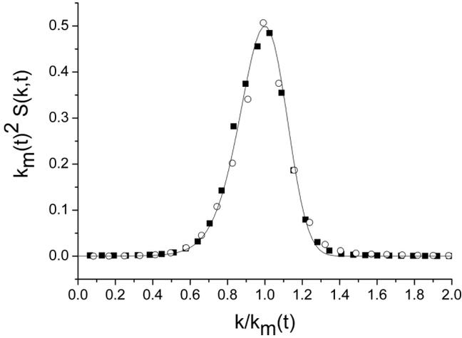
FIG. 1. Comparison between  $S(k,t)$  derived from our ansatz (full line) and extracted from numerical simulations of Eq. (2) (black squares and open circles). Computations were performed in two dimensions ( $d = 2$ ) using a finite difference scheme in the Fourier space with a  $512 \times 512$  grid size for large times [the reduced times were equal to 2000 (black squares) and 5000 (open circles); for each time, simulations were averaged over 100 random initial configurations].
