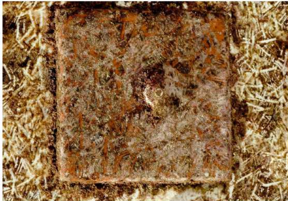
Fig. 5. Tile immersed for 3 mo, showing typical Scaridae bite marks
