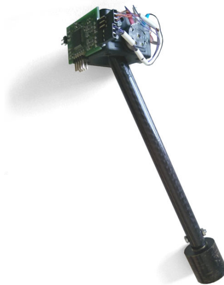
Figure 7.21 – The pendulum. The load orientation PCB is on the left side of the basis. One of the potentiometers is on the right side of the basis. The other is hidden, on the side opposite to the PCB.
