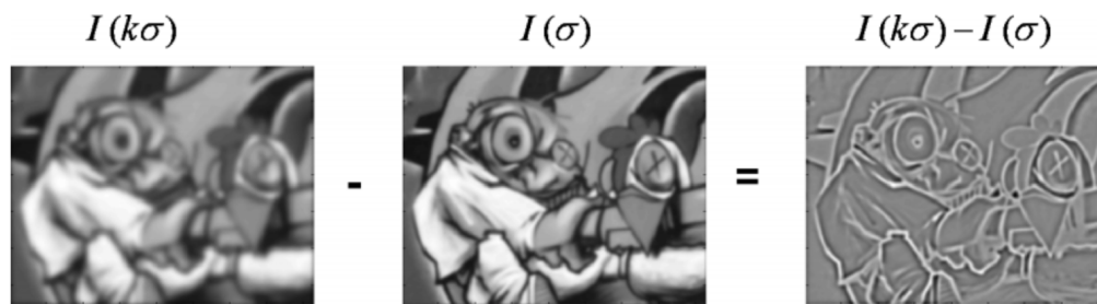
Figure 2.6 – The Laplacian-of-Gaussian can be approximated as a difference of two Gaussian smoothed images, source: [Tuytelaars 08]
