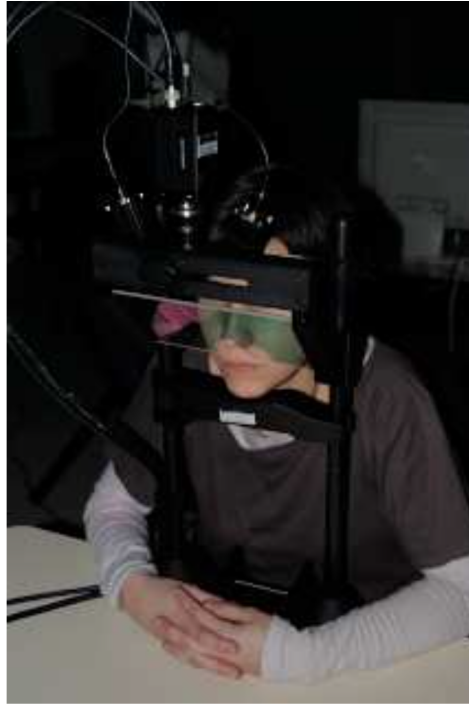
Figure 3.7 – Eye-tracker from Cambridge Research Ltd (picture from [Boujut 12b])
