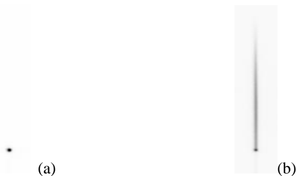
Figure 3.16: The correct image (a) and the wrong image (b) due to the streaking (the color is inverted)
