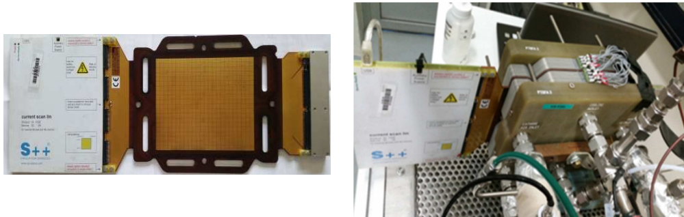
Figure II.14 : Sensor plate out of the stack and inserted in the middle of the stack
