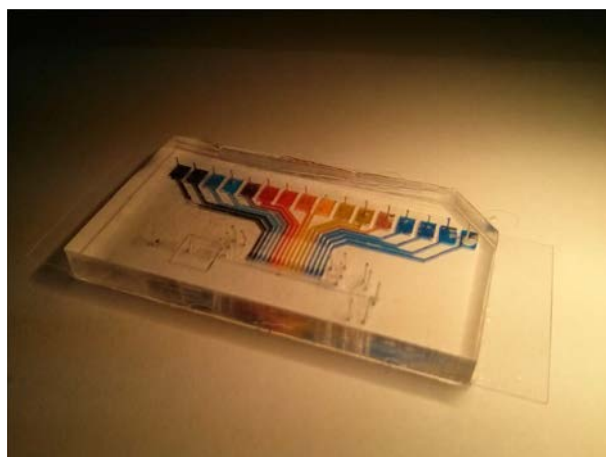
Figure 7.8 – Multiplexed platform for the in situ encoding of droplets with DNA barcodes
