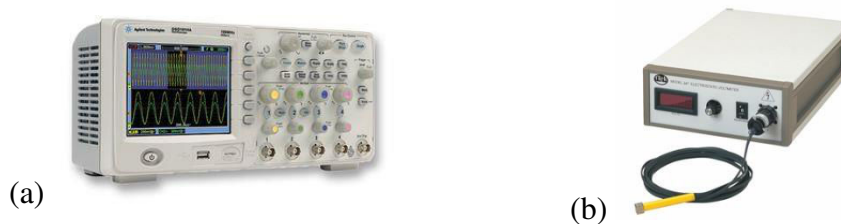
Figure 4.2. (a) oscilloscope Agilent Technologies DSO1014A, (b) non-contacting electrostatic voltmeter TREK 370.
