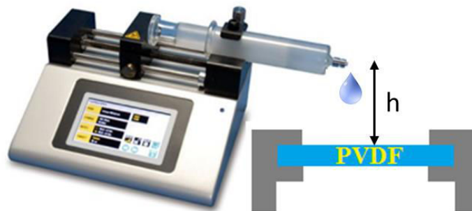
Figure 4.4. Schematic representation of water drop experiment (not to scale).
