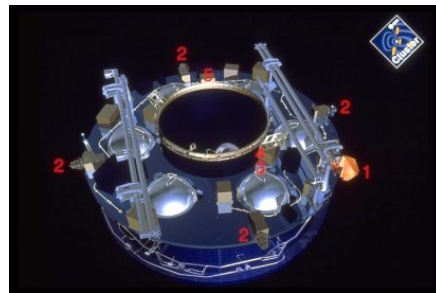
FIGURE 3.3: Cutaway of Cluster spacecraft main equipment platform, showing the STAFF (1), EFW (2), DWP (3), WHISPER (4) and WBD (5) instruments.
