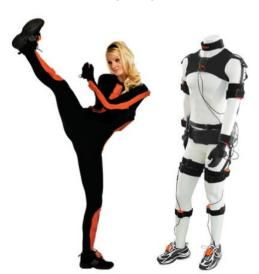
the body (See Figure 3.1). Many cameras are mostly used to track the markers position. The use of more cameras is appreciated to deal with occlusion problems. The Vicon motion capture system is one of the most well known optical motion capture systems [Roether et al., 2009] [Hicheur et al., 2013] [Busso et al., 2008]. While providing accurate motion capture data, advanced computer vision techniques are required to track the markers positions.
