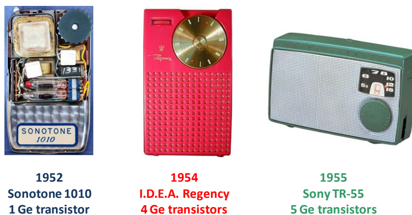
Figure IV-3: The first marketed transistorized products in the early 1950's contained Germanium transistors.
