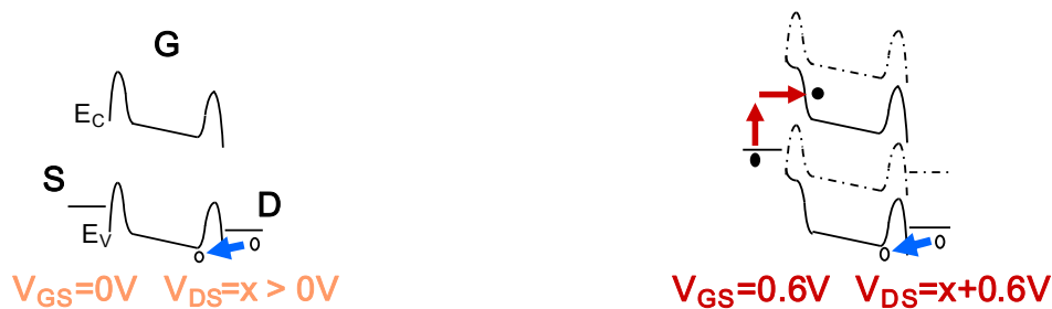
Figure III-10: Schematic cross-sectional band diagrams in the channel direction under nFET bias at a given positive V_{DS} bias x with V_{GS}=0V (left) and at V_{DS}=x+0.6V ; V_{GS}=0.6V (right). The dashed lines on the right are reminiscent of the bands configuration on the left.
