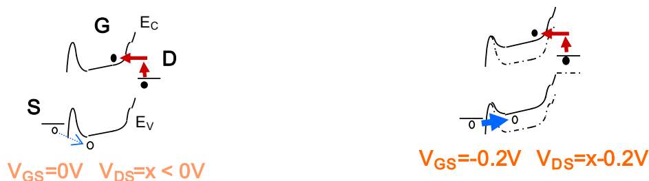
Figure III-9: Schematic cross-sectional band diagrams in the channel direction under pFET bias at a given negative V_{DS} bias x with V_{GS}=0\text{V} (left) and at V_{DS}=x-0.2\text{V} ; V_{GS}=-0.2\text{V} (right). The dashed lines on the right are reminiscent of the bands configuration on the left.
