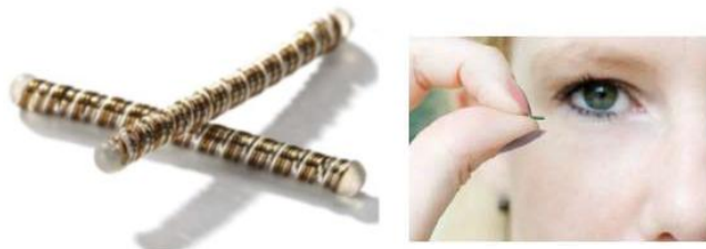
Figure 9: Tear drop micro glucose sensor (NovioSense™). [55]
