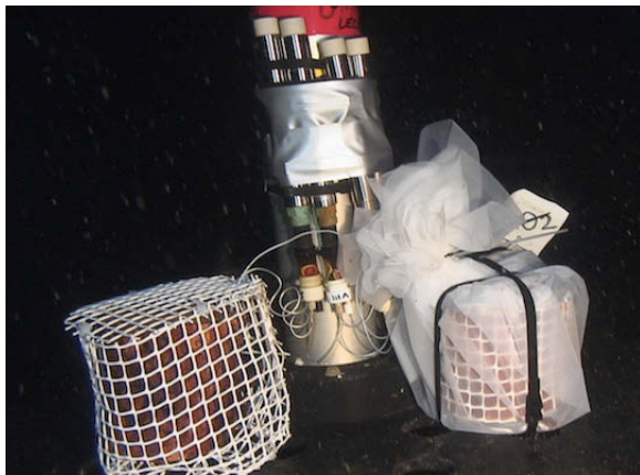
Supplementary figure 1 An unprotected cage (left) and a mesh protected cage (right) equipped with hydrogen sulphide sensors. The picture was taken by the R.O.V. Super Achille at 520m depth in the Lacaze-Duthiers submarine canyon at the beginning of the experiment.
