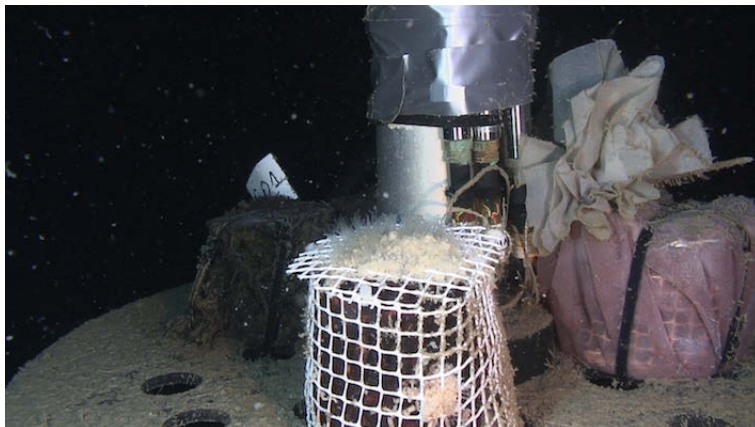
Supplementary figure 2 An unprotected cage (left) and a mesh protected cage (right) equipped with hydrogen sulphide sensors after 85 days of immersion in the Lacaze-Duthiers submarine canyon.
