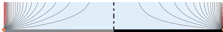
FIGURE 2.23 – Left : Isolines for the radial velocity \tilde{u}_r extracted from the numerical simulations. Right : Theoretical isolines for the radial velocity given by the composite expansion \tilde{u}_r^{\text{comp}} . Note that the transverse scale has here been stretched to visualize the boundary layer.
