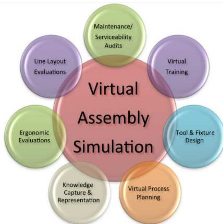
Figure 2.1 Applications of a virtual assembly/disassembly simulation [Set 11]
