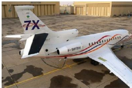
Figure 1. Falcon 7X. Transition has been measured on the horizontal tail plane by infra-red measurements. The zone of interest is colored in black.
