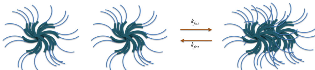
Figure 4.2. Schematic representation of fusion and fission of complete micelles, where k_{fus} corresponds to the kinetic constant of the fusion process and k_{fra} corresponds to the kinetic constant of the fission process [22].
