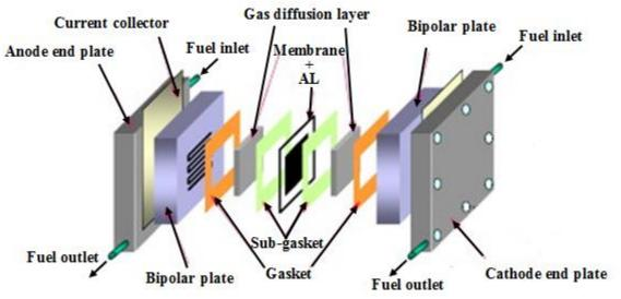
Fig. 2. Scheme of a unit fuel cell assembly [8].
