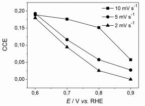
Fig. 23. CO<sub>2</sub> current efficiency (CCE) values calculated from cyclic voltammetries run in 0.5 M  $H_2SO_4 + 0.1$  M EtOH (represented in Fig. 22a) at v = 2, 5 and 10 mV s<sup>-1</sup> and corresponding MSCVs (Fig. 22b) on Pt/C.
