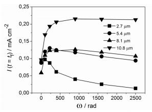
Fig. 20. Evolution of the potentiostatic current (CA at E = 0.7 V vs. RHE) recorded at  $t_f = 630$  s against the rotation speed.
