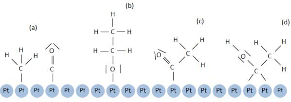
Fig. 4. Adsorption modes of ethanol adsorbates on Pt.
