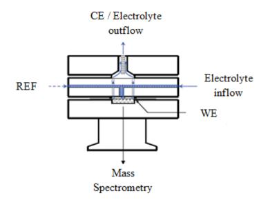
Fig. 10. Scheme of the electrochemical DEMS flow cell [160].
