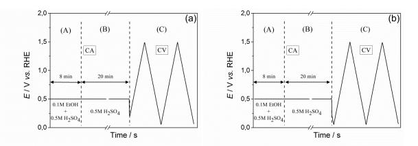
Fig. 55. Potential *vs.* time representation of (A) the adsorbates adsorption in 0.5 M  $H_2SO_4 + 0.1$  M EtOH (represented here at  $E_{ad} = 0.5$  V *vs.* RHE), (B) the flush of the solution in 0.5 M  $H_2SO_4$  and (C) the adsorbates electrooxidation starting at E = 0.2 V *vs.* RHE with a first (a) positive (hereafter noted "direct") and (b) negative (hereafter noted "indirect") sweep.
