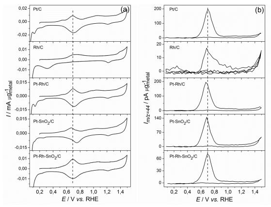
Fig. 69. (a) CV of the electrooxidation of ethanol adsorbates in 0.5 M H<sub>2</sub>SO<sub>4</sub> after adsorption at  $E_{ad} = 0.3$  V vs. RHE and the corresponding MSCV for mass-to-charge ratio (b) m/z = 44 on Pt/C, Rh/C, Pt-Rh/C, Pt-SnO<sub>2</sub>/C and Pt-Rh-SnO<sub>2</sub>/C; v = 10 mV s<sup>-1</sup>;  $T = 25^{\circ}$ C.
