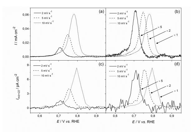
Fig. 21. Substracted (a) non-amplified and (b) amplified CO-stripping CVs in 0.5 M H<sub>2</sub>SO<sub>4</sub> on Pt/C (metal loading: 9.9 µg) and corresponding (c) non-amplified and (d) amplified MSCVs for mass-to-charge ratio m/z = 22 multiplied by a number indicated in brackets;  $T = 25^{\circ}$ C.
