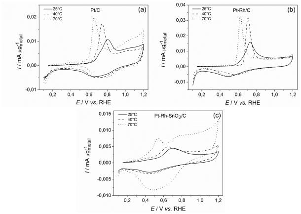
Fig. 78. CO-stripping CV in 0.5 M H<sub>2</sub>SO<sub>4</sub> on (a) Pt/C, (b) Pt-Rh/C and (c) Pt-Rh-SnO<sub>2</sub>/C;  $T = 25^{\circ}$ C (full), 40°C (dash) and 70°C (dots);  $v = 10 \text{ mV s}^{-1}$ .
