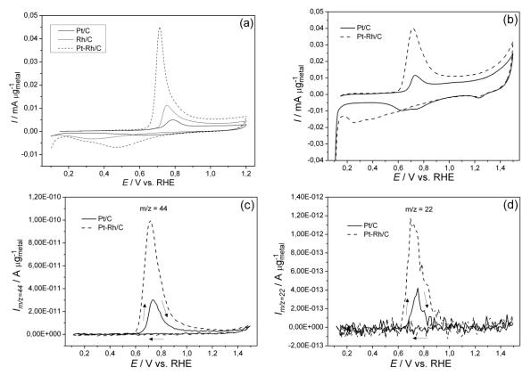
Fig. 83. CO-stripping CV in 0.5 M H2SO4 in (a) static and (b) flow electrolyte and corresponding MSCV for mass to charge ratio (c) m/z = 44 and (d) m/z = 22 of the CO stripping on (solid) Pt/C and (dash) Pt-Rh/C; v = 10 mV s<sup>-1</sup>;  $T = 25^{\circ}$ C.
