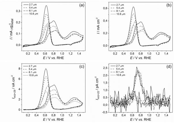
Fig. 15. (a) CV of the EOR in 0.5 M H<sub>2</sub>SO<sub>4</sub> + 0.1 M EtOH on Pt/C (L = 2.7, 5.4, 8.1 and 10.8  $\mu$ m) normalized by the (a) metal loading and (b) ECSA and corresponding MSCV for mass-to-charge ratio (c) m/z = 29 and (d) m/z = 22 (normalized by the ECSA); v = 10 mV s<sup>-1</sup>;  $T = 25^{\circ}$ C.
