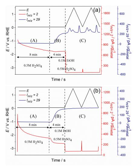
Fig. 47. Evolution of the potential and mass-to-charge ratio signals m/z = 2 and m/z = 29 vs. time on (a) Pt/C and (b) Rh/C during three consecutive steps: (A) hydrogen adsorption in 0.5 M H<sub>2</sub>SO<sub>4</sub> at  $E_{ad} = 0.05$  V vs. RHE, (B) the solution change in 0.5 M H<sub>2</sub>SO<sub>4</sub> + 0.1 M EtOH and (C) the potentiodynamic ethanol oxidation reaction starting at E = 0.2 V vs. RHE.
