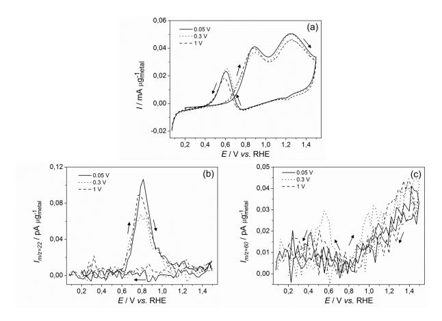
Fig. 52. (a) CV of the EOR in 0.5 M H<sub>2</sub>SO<sub>4</sub> + 0.1 M acetaldehyde after adsorption at  $E_{ad} = 0.05$  (solid), 0.3 (dots) and 1 V vs. RHE (dash) and corresponding MSCV for mass-to-charge ratio (b) m/z = 22 and (c) m/z = 60 on Pt-Rh/C; v = 10 mV s<sup>-1</sup>;  $T = 25^{\circ}$ C.
