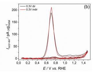
Fig. 59. (a) CV of the electrooxidation of ethanol adsorbates in 0.5 M H<sub>2</sub>SO<sub>4</sub> after adsorption at  $E_{ad} = 0.3$  V vs. RHE (black) without and (red) with a first reduction scan and the corresponding MSCV for mass-to-charge ratio (b) m/z = 44 on Pt/C; v = 10 mV s<sup>-1</sup>;  $T = 25^{\circ}$ C.
