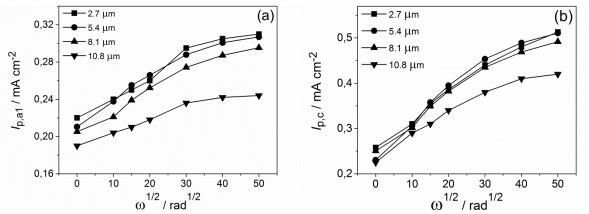
Fig. 18. Evolution of the peak current between (a) E = 0.3 and 1 V vs. RHE and (b) E = 0.8 and 0.4 V vs. RHE against the rotation speed.
