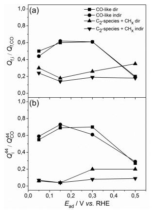
Fig. 63. Relative coverage of the Pt/C surface by acetaldehyde adsorbates adsorbed at  $E_{ad} = 0.05, 0.15, 0.3$  and 0.5 V vs.RHE deduced from (a) faraday charges and (b) ionic charges from the mass-to-charge signal m/z = 44.
