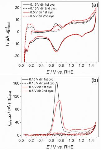
Fig. 60. (a) CV of the electrooxidation of ethanol adsorbates in 0.5 M H<sub>2</sub>SO<sub>4</sub> after adsorption at (black)  $E_{ad} = 0.15$  V vs. RHE and (red)  $E_{ad} = 0.5$  V vs.RHE and the corresponding MSCV for mass-to-charge ratio (b) m/z = 44 on Pt/C; v = 10 mV s<sup>-1</sup>;  $T = 25^{\circ}$ C.
