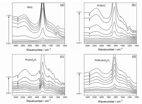
Fig. 34. *In situ* infrared spectra recorded in 0.5M  $H_2SO_4 + 0.1M$  EtOH on (a) Rh/C, (b) Pt-Rh/C, (c) Pt-SnO<sub>2</sub>/C and (d) Pt-Rh-SnO<sub>2</sub>/C at room temperature;  $R_{ref} = 0.15$  V vs. RHE. Potential range: E = 0.25 and 1.15 V vs. RHE; Potential step: E = 0.1 V.
