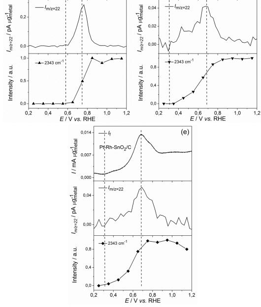
Fig. 31. CO-stripping CV in 0.5 M H<sub>2</sub>SO<sub>4</sub>, corresponding MS signal m/z = 22 and CO<sub>2</sub> band intensity (from Fig. 30) on (a) Pt/C, (b) Rh/C, (c) Pt-Rh/C, (d) Pt-SnO<sub>2</sub>/C and (e) Pt-Rh-SnO<sub>2</sub>/C; v = 10 mV s<sup>-1</sup>;  $T = 25^{\circ}$ C.
