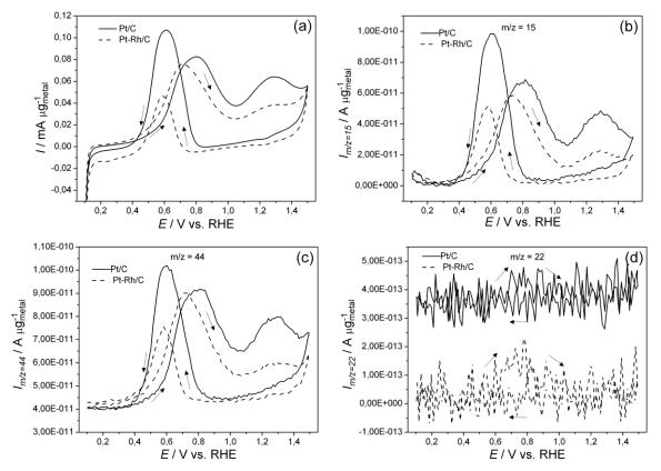
Fig. 84. (a) CV in 0.5 M H<sub>2</sub>SO<sub>4</sub> + 0.1 M EtOH and MSCV for mass to charge ratio (b) m/z = 15, (c) m/z = 44 and (d) m/z = 22 of the EOR on (solid) Pt/C and (dash) Pt-Rh/C; v = 10 mV s<sup>-1</sup>;  $T = 25^{\circ}$ C.
