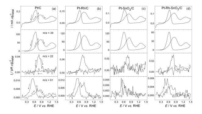
Fig. 45. CV of the EOR in 0.5 M H<sub>2</sub>SO<sub>4</sub> + 0.1 M EtOH after adsorption at  $E_{ad} = 0.05$  on (a) Pt/C, (b) Pt-Rh/C, (c) Pt-SnO<sub>2</sub>/C and (d) Pt-Rh-SnO<sub>2</sub>/C and corresponding MSCV for mass-to-charge ratio m/z = 29, m/z = 22 and m/z = 61; v = 10 mV s<sup>-1</sup>;  $T = 25^{\circ}$ C.
