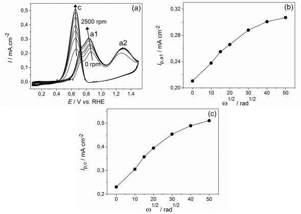
Fig. 14. (a) CV in 0.5 M H<sub>2</sub>SO<sub>4</sub> + 0.1 EtOH on Pt/C (metal loading: 9.9 µg) on a RDE at different rotation speeds: 0, 100, 225, 400, 900, 1600, 2500 rpm; Evolution of the peak current between (b) E = 0.3 and 1 V vs. RHE ( $I_{p,a1}$ ) and between (c) E = 0.8 and 0.4 V vs. RHE ( $I_{p,c}$ ) against the rotation speed; v = 10 mV s<sup>-1</sup>;  $T = 25^{\circ}$ C.
