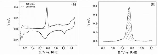
Fig. 8. (a) 1<sup>st</sup> (solid) and 2<sup>nd</sup> cycle (dash) of a CO stripping CV in 0.5 M H<sub>2</sub>SO<sub>4</sub> in the DEMS flow cell and associated (b) substraction of the 1<sup>st</sup> cycle by the 2<sup>nd</sup> one.
