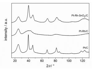
Fig. 75. XRD pattern of 10wt.% carbon supported Pt/C, Pt-Rh/C and Pt-Rh-SnO<sub>2</sub>/C electrocatalysts prepared by the polyol method.
