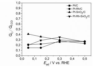
Fig. 71. Relative coverage of Pt/C, Pt-Rh/C, Pt-SnO<sub>2</sub>/C and Pt-Rh-SnO<sub>2</sub>/C electroactive surface by "strong ethanol adsorbates" (oxidizing at E > 0.9 V vs. RHE) adsorbed at  $E_{ad} = 0.05, 0.15, 0.3$  and 0.5 V vs. RHE deduced from faraday charges.
