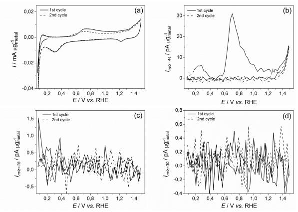
Fig. 68. (a) CV of the electrooxidation of ethanol adsorbates in 0.5 M H<sub>2</sub>SO<sub>4</sub> after adsorption at  $E_{ad} = 0.3$  V vs. RHE with a first reduction scan and the corresponding MSCV for mass-to-charge ratio (b) m/z = 44, (c) m/z = 15 and (d) m/z = 30 on Rh/C; v = 10 mV s<sup>-1</sup>;  $T = 25^{\circ}$ C.
