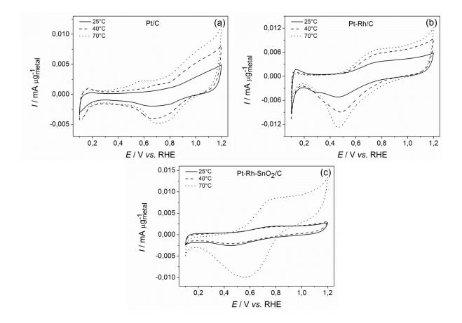
Fig. 77. CV in 0.5 M H<sub>2</sub>SO<sub>4</sub> on (a) Pt/C, (b) Pt-Rh/C and (c) Pt-Rh-SnO<sub>2</sub>/C at  $T = 25^{\circ}$ C (full), 40°C (dash) and 70°C (dots);  $v = 10 \text{ mV s}^{-1}$ .
