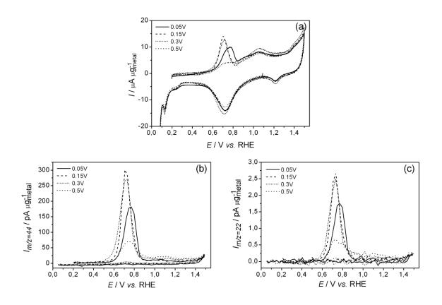
Fig. 62. (a) CV of the electrooxidation of acetaldehyde adsorbates in 0.5 M H<sub>2</sub>SO<sub>4</sub> after adsorption at  $E_{ad} = 0.05$  (solid), 0.15 (dash), 0.3 (short dash) and 0.5 V vs. RHE (dots) and corresponding MSCV for mass-to-charge ratio (b) m/z = 44 and (c) m/z = 22 on Pt/C; v = 10 mV s<sup>-1</sup>;  $T = 25^{\circ}$ C.
