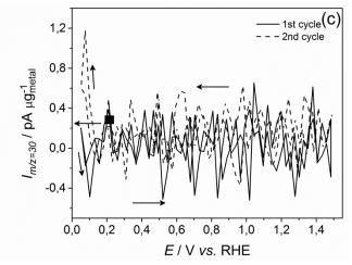
Fig. 66. (a) CV and related MSCV of the electrooxidation of acetaldehyde adsorbates in 0.5 M H<sub>2</sub>SO<sub>4</sub> after adsorption at  $E_{ad} = 0.05$  V vs. RHE with a first reduction scan for the mass-tocharge ratio (b) m/z = 15 and (c) m/z = 30 on Pt/C; (solid) 1<sup>st</sup> and (dash) 2<sup>nd</sup> cycle; v = 10 mV s<sup>-1</sup>;  $T = 25^{\circ}$ C.
