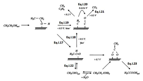
Fig. 3. Scheme of the ethanol oxidation reaction [21].
