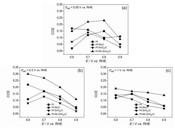
Fig. 46. Potentiodynamic EOR CO<sub>2</sub> current efficiency (CCE) values deduced from cyclic voltammetries in 0.5 M H<sub>2</sub>SO<sub>4</sub> + 0.1 M EtOH on Pt/C, Pt-Rh/C, Pt-SnO<sub>2</sub>/C and Pt-Rh-SnO<sub>2</sub>/C preceded by CA at  $E_{ad} = (a) 0.05$ , (b) 0.3 and (c) 1 V vs. RHE.
