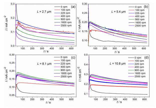
Fig. 19. CA on a RDE at different rotation speeds ( $\omega = 0$ , 100, 225, 400, 900, 1600 and 2500 rpm) in 0.5 M H<sub>2</sub>SO<sub>4</sub> + 0.1 EtOH on Pt/C at different thickness layers: L = (a) 2.7, (b) 5.4, (c) 8.1 and (d) 10.8 µm; v = 10 mV s<sup>-1</sup>;  $T = 25^{\circ}$ C.
