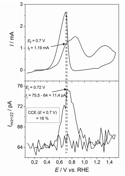
Fig. 12. EOR CCE calculation at E = 0.7 V vs. RHE in 0.5 M H<sub>2</sub>SO<sub>4</sub> + 0.1 M EtOH.
