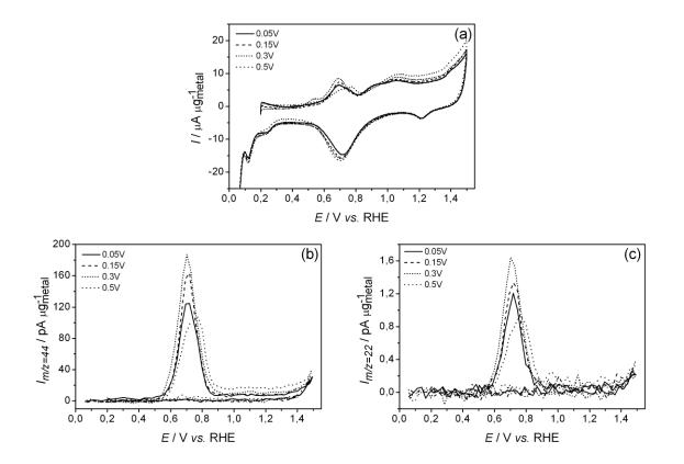
Fig. 56. (a) CV of the electrooxidation of ethanol adsorbates in 0.5 M H<sub>2</sub>SO<sub>4</sub> after adsorption at  $E_{ad} = 0.05$  (solid), 0.15 (dash), 0.3 (short dash) and 0.5 V vs. RHE (dots) and corresponding
