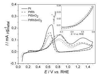
Fig. 44. (a) CV of the EOR in 0.5 M H<sub>2</sub>SO<sub>4</sub> + 0.1 M EtOH after CA at  $E_{ad} = 0.05$  V vs. RHE on Pt/C (solid), Pt-Rh/C (dash), Pt-SnO<sub>2</sub>/C (dots) and Pt-Rh-SnO<sub>2</sub>/C (short dots); v = 10 mV s<sup>-1</sup>;  $T = 25^{\circ}$ C.
