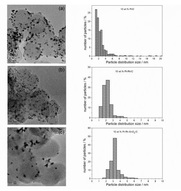
Fig. 76. Typical TEM images and associated particle size distribution of the 10 wt. % (a) Pt/C, (b) Pt-Rh/C and (c) Pt-Rh-SnO<sub>2</sub>/C electrocatalysts.
