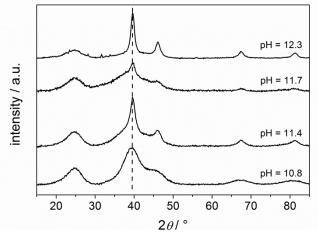
Fig. 13. XRD pattern of the carbon supported Pt/C electrocatalysts prepared by Polyol method at pH = 12.3, 11.7, 11.3 and 10.7.
