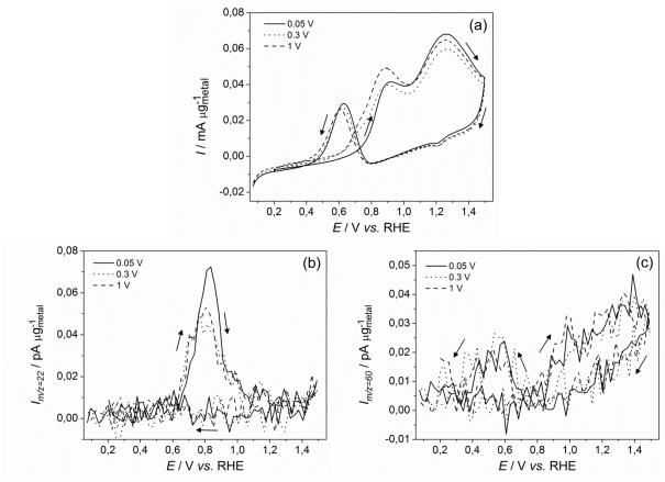
Fig. 53. (a) CV of the EOR in 0.5 M H<sub>2</sub>SO<sub>4</sub> + 0.1 M acetaldehyde after adsorption at  $E_{ad} = 0.05$  (solid), 0.3 (dots) and 1 V vs. RHE (dash) and corresponding MSCV for mass-to-charge ratio (b) m/z = 22 and (c) m/z = 60 on Pt-Rh-SnO<sub>2</sub>/C; v = 10 mV s<sup>-1</sup>;  $T = 25^{\circ}$ C.
