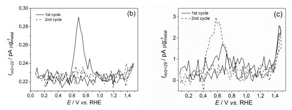
Fig. 42. (solid) First and (dash) second scan of the (a) potentiodynamic EOR in 0.5 M H<sub>2</sub>SO<sub>4</sub> + 0.1 M EtOH after adsorption at  $E_{ad} = 0.05$  V vs. RHE and corresponding MSCV for mass-to-charge ratio (b) m/z = 22 and (c) m/z = 29 on Rh/C; v = 10 mV s<sup>-1</sup>;  $T = 25^{\circ}$ C.
