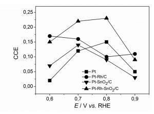
Fig. 37. (a) EOR CO<sub>2</sub> current efficiency (CCE) values calculated from cyclic voltammetries run in 0.5 M H<sub>2</sub>SO<sub>4</sub> + 0.1 M EtOH (represented in Fig. 33 and Fig. 36) and corresponding MSCVs (in Fig. 33 and Fig. 36) on Pt/C, Pt-Rh/C, Pt-SnO<sub>2</sub>/C and Pt-Rh-SnO<sub>2</sub>/C.
