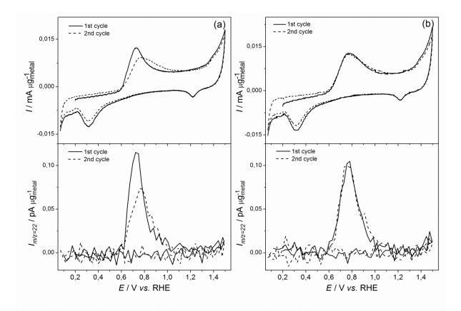
Fig. 51. (solid) First and (dash) second scan of the potentiodynamic acetaldehyde in 0.5 M  $H_2SO_4 + 0.1$  M acetaldehyde after adsorption at  $E_{ad} = (a) 0.05$  and (b) 1 V vs. RHE and corresponding MSCV for mass-to-charge ratio m/z = 22 on Rh/C; v = 10 mV s<sup>-1</sup>;  $T = 25^{\circ}$ C.
