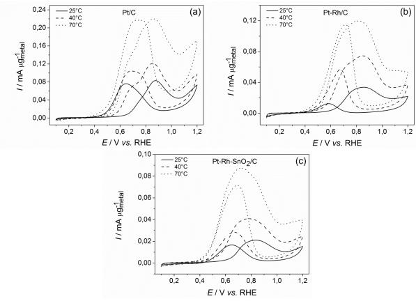
Fig. 79. CV in 0.5 M H<sub>2</sub>SO<sub>4</sub> + 0.1 M EtOH of the EOR on (a) Pt/C, (b) Pt-Rh/C and (c) Pt-Rh-SnO<sub>2</sub>/C;  $T = 25^{\circ}$ C (solid), 40°C (dash) and 70°C (dots);  $v = 10 \text{ mV s}^{-1}$ .
