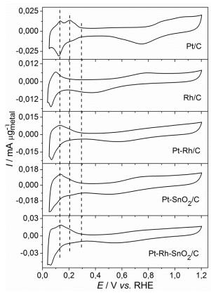
Fig. 26. CV in 0.5 M H<sub>2</sub>SO<sub>4</sub> on Pt/C, Rh/C, Pt-Rh/C, Pt-SnO<sub>2</sub>/C and Pt-Rh-SnO<sub>2</sub>/C electrocatalysts;  $v = 10 \text{ mV s}^{-1}$ ;  $T = 25^{\circ}$ C.
