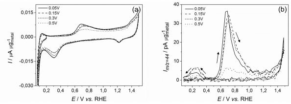
Fig. 67. (a) CV of the electrooxidation of ethanol adsorbates in 0.5 M H<sub>2</sub>SO<sub>4</sub> after adsorption at  $E_{ad} = 0.05$  (solid), 0.15 (dash), 0.3 (short dash) and 0.5 V vs. RHE (dots) and corresponding MSCV for mass-to-charge ratio (b) m/z = 44 and on Rh/C; v = 10 mV s<sup>-1</sup>;  $T = 25^{\circ}$ C.
