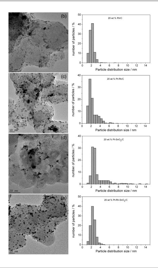
Fig. 25. Typical TEM images at × 200 000 magnification and associated particle size distribution of the (a) Pt/C, (b) Rh/C, (c) Pt-Rh/C, (d) Pt-SnO<sub>2</sub>/C and (e) Pt-Rh-SnO<sub>2</sub>/C electrocatalysts.
