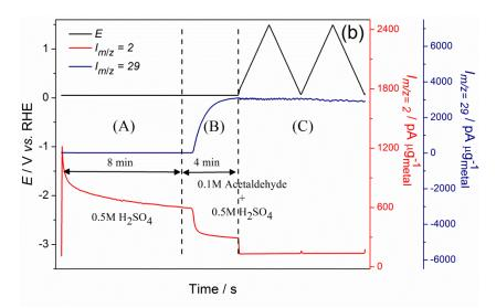
Fig. 54. Evolution of the potential and mass-to-charge ratio signals m/z = 2 and m/z = 29 vs. time on (a) Pt/C and (b) Pt-SnO<sub>2</sub>/C during three consecutive steps: (A) hydrogen adsorption in
