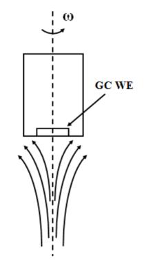
Fig. 7. Flow profile at a rotating disc electrode (RDE).
