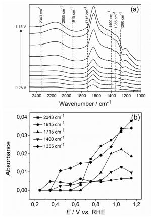
Fig. 32. (a) *In situ* infrared spectra recorded in 0.5M H<sub>2</sub>SO<sub>4</sub> + 1M EtOH on Pt/C at room temperature and (b) band intensities evolution (at 2343, 1915, 1715, 1400 and 1355 cm<sup>-1</sup>) against the applied potential;  $R_{ref} = 0.15$  V vs. RHE. Potential range: E = 0.25 and 1.15 V vs. RHE; Potential step: E = 0.1 V.
