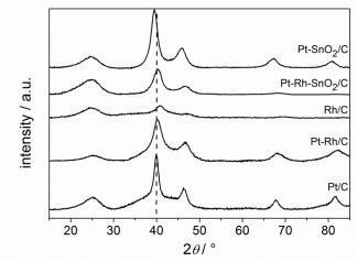
Fig. 24. XRD pattern of carbon supported 20 wt.% Pt/C, Rh/C, Pt-Rh/C, Pt-SnO<sub>2</sub>/C and Pt-Rh-SnO<sub>2</sub>/C electrocatalysts prepared by Polyol method.
