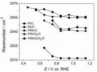
Fig. 29. Variation of the CO<sub>L</sub> band wavenumber *versus* potential, measured during the CO stripping in 0.5 M H<sub>2</sub>SO<sub>4</sub> on Pt/C, Rh/C, Pt-Rh/C, Pt-SnO<sub>2</sub>/C and Pt-Rh-SnO<sub>2</sub>/C;  $T = 25^{\circ}$ C.
