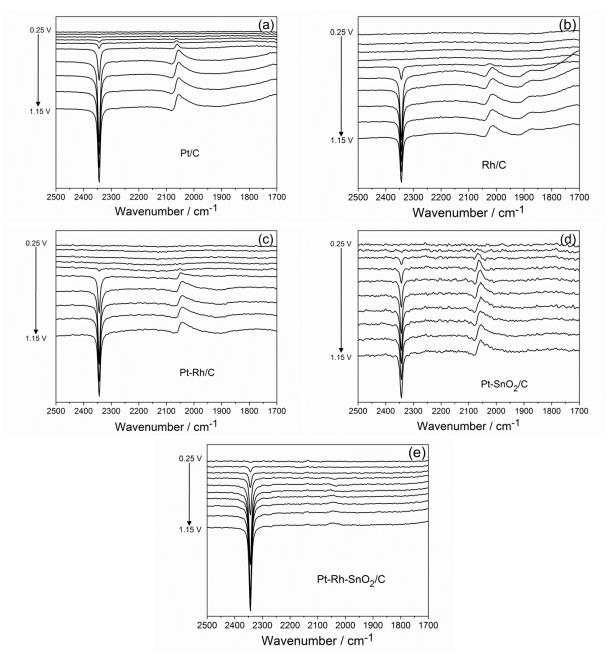
Fig. 28. *In situ* infrared spectra recorded during CO stripping in 0.5 M H<sub>2</sub>SO<sub>4</sub> on (a) Pt/C, (b) Rh/C, (c) Pt-Rh/C, (d) Pt-SnO<sub>2</sub>/C and (e) Pt-Rh-SnO<sub>2</sub>/C;  $T = 25^{\circ}$ C.
