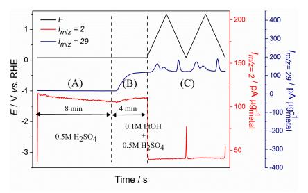
Fig. 48. Evolution of the potential and mass-to-charge ratio signals m/z = 2 and m/z = 29 vs. time on Pt-Rh-SnO<sub>2</sub>/C during three consecutive steps: (A) hydrogen adsorption in 0.5 M H<sub>2</sub>SO<sub>4</sub> at  $E_{ad} = 0.07$  V vs. RHE, (B) the solution change in 0.5 M H<sub>2</sub>SO<sub>4</sub> + 0.1 M EtOH and
