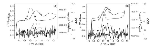
Fig. 85. EOR CV in 0.5 M  $H_2SO_4 + 0.1$  M EtOH, MSCV for mass to charge ratio m/z = 22 and (line + symbol) CCE of the EOR on (left) Pt/C and (right) Pt-Rh/C.
