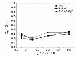
Fig. 74. Relative coverage of Pt/C, Pt-Rh/C and Pt-Rh-SnO<sub>2</sub>/C electroactive surface by "strong acetalehyde adsorbates" (oxidizing at E > 0.9 V vs. RHE) adsorbed at  $E_{ad} = 0.05$ , 0.15, 0.3 and 0.5 V vs. RHE deduced from faraday charges.
