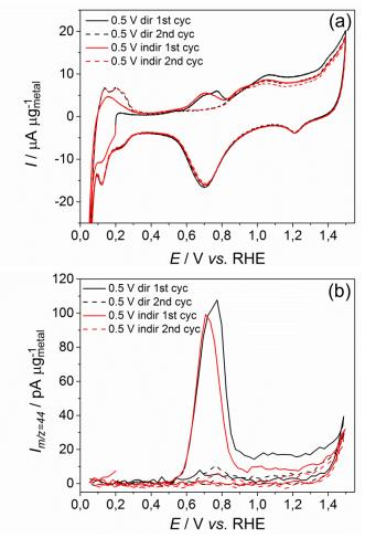
Fig. 61. (a) CV of the electrooxidation of ethanol adsorbates in 0.5 M H<sub>2</sub>SO<sub>4</sub> after adsorption at  $E_{ad} = 0.5$  V vs. RHE without a first reduction scan (black) and with a first reduction scan (red) and the corresponding MSCV for mass-to-charge ratio (b) m/z = 44 on Pt/C; v = 10 mV s<sup>-1</sup>;  $T = 25^{\circ}$ C.
