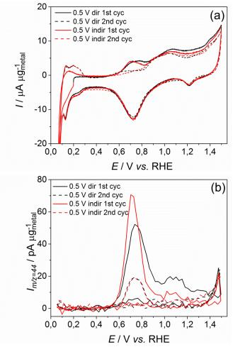
Fig. 65. (a) CV of the electrooxidation of acetaldehyde adsorbates in 0.5 M H<sub>2</sub>SO<sub>4</sub> after adsorption at  $E_{ad} = 0.5$  V vs. RHE (black) without and (red) with a first reduction scan and the corresponding MSCV for mass-to-charge ratio (b) m/z = 44 on Pt/C; v = 10 mV s<sup>-1</sup>;  $T = 25^{\circ}$ C.
