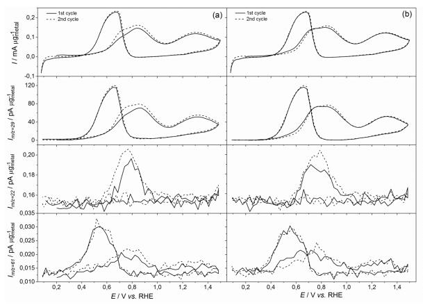
Fig. 40. (solid) First and (dash) second scan of the potentiodynamic EOR in 0.5 M H<sub>2</sub>SO<sub>4</sub> + 0.1 M EtOH after adsorption at  $E_{ad} =$  (a) 0.05 and (b) 1 V vs. RHE and corresponding MSCV for mass-to-charge ratio m/z = 44, m/z = 22 and m/z = 61 on Pt/C; v = 10 mV s<sup>-1</sup>;  $T = 25^{\circ}$ C.
