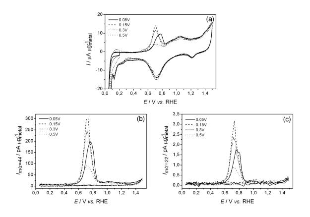
Fig. 64. (a) CV of the electrooxidation of acetaldehyde adsorbates in 0.5 M H<sub>2</sub>SO<sub>4</sub> after adsorption at  $E_{ad} = 0.05$  (solid), 0.15 (dash), 0.3 (short dash) and 0.5 V vs. RHE (dots) and corresponding MSCV for mass-to-charge ratio (b) m/z = 44 and (c) m/z = 22 on Pt/C; v = 10 mV s<sup>-1</sup>;  $T = 25^{\circ}$ C.
