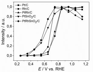
Fig. 30. (a) CO stripping in 0.5 M H<sub>2</sub>SO<sub>4</sub> - CO<sub>2</sub> band intensity against potentials on Pt/C, Rh/C, Pt-Rh/C, Pt-SnO<sub>2</sub>/C and Pt-Rh-SnO<sub>2</sub>/C;  $T = 25^{\circ}$ C.
