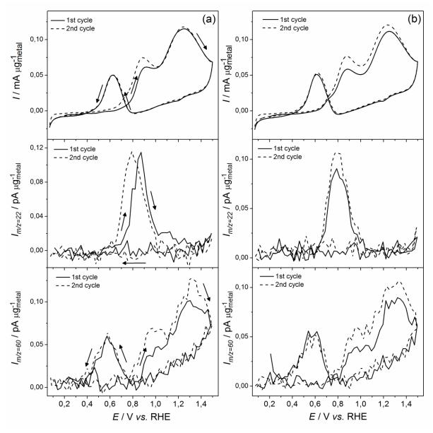
Fig. 50. (solid) First and (dash) second scan of the potentiodynamic acetaldehyde in 0.5 M  $H_2SO_4 + 0.1$  M acetaldehyde after adsorption at  $E_{ad} = (a) 0.05$  and (b) 1 V vs. RHE and corresponding MSCV for mass-to-charge ratio m/z = 22 and m/z = 60 on Pt/C; v = 10 mV s<sup>-1</sup>;  $T = 25^{\circ}C$ .
