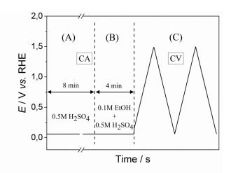
Fig. 38. Potential *vs*. time representation of (A) the adsorbates adsorption in 0.5 M H<sub>2</sub>SO<sub>4</sub> (represented here at  $E_{ad} = 0.05$  V *vs*. RHE), (B) the solution change in 0.5 M H<sub>2</sub>SO<sub>4</sub> + 0.1 M EtOH and (C) the potentiodynamic ethanol oxidation reaction starting at E = 0.2 V *vs*. RHE.
