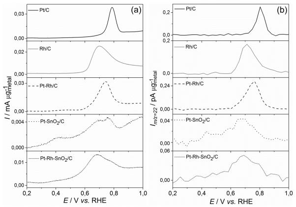
Fig. 27. (a) CO-stripping CV in 0.5 M H<sub>2</sub>SO<sub>4</sub> in and (b) corresponding MSCV for mass to charge ratio m/z = 22 on Pt/C, Rh/C, Pt-Rh/C, Pt-SnO2/C and Pt-Rh-SnO<sub>2</sub>/C; v = 10 mV s<sup>-1</sup>;  $T = 25^{\circ}$ C.
