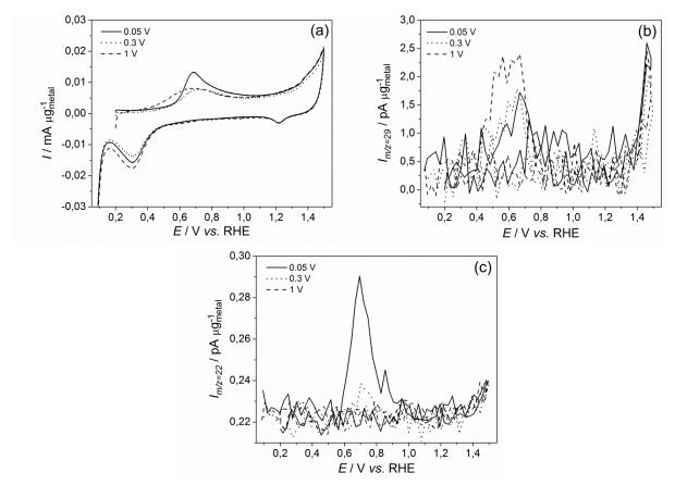
Fig. 41. (a) CV of the EOR in 0.5 M H<sub>2</sub>SO<sub>4</sub> + 0.1 M EtOH after adsorption at  $E_{ad} = 0.05$  (solid), 0.3 (dots) and 1 V vs. RHE (dash) and corresponding MSCV for mass-to-charge ratio (b) m/z = 29, (c) m/z = 22 on Rh/C; v = 10 mV s<sup>-1</sup>;  $T = 25^{\circ}$ C.
