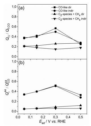
Fig. 58. Relative coverage of the Pt/C surface by ethanol adsorbates adsorbed at  $E_{ad} = 0.05$ , 0.15, 0.3 and 0.5 V vs. RHE deduced from (a) faraday charges and (b) ionic charges from the mass-to-charge signal m/z = 44.
