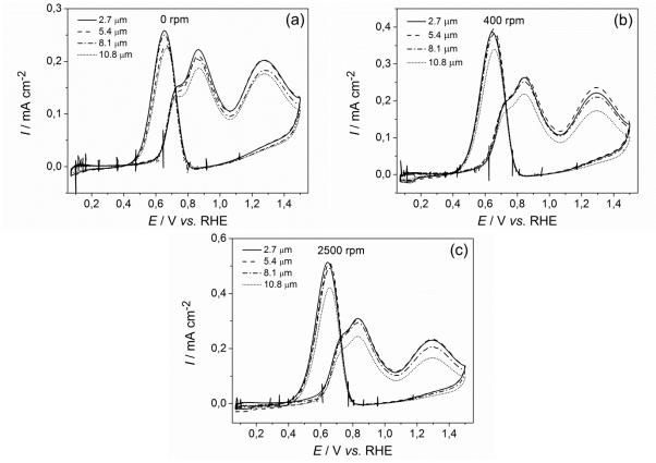
Fig. 17. CV in 0.5 M H<sub>2</sub>SO<sub>4</sub> + 0.1 EtOH on Pt/C (L = 2.7, 5.4, 8.1 and 10.8 µm) on a RDE at different rotation speeds:  $\omega = (a) 0$ , (b) 400 and (c) 2500 rpm;  $v = 10 \text{ mV s}^{-1}$ ;  $T = 25^{\circ}$ C.
