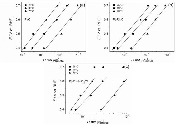
Fig. 80. Tafel plots of potentiostatic currents recorded after 900 s at potentials from 0.4 to 0.7 V vs. RHE (0.1 V step) in 0.5 M  $H_2SO_4 + 0.1$  M EtOH on (a) Pt/C, (b) Pt-Rh/C and (c) Pt-Rh-SnO<sub>2</sub>/C at 25°C, 40°C and 70°C.
