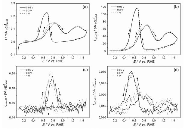
Fig. 39. (a) CV of the EOR in 0.5 M H<sub>2</sub>SO<sub>4</sub> + 0.1 M EtOH after adsorption at  $E_{ad} = 0.05$  (solid), 0.3 (dots) and 1 V vs. RHE (dash) and corresponding MSCV for mass-to-charge ratio (b) m/z = 29, (c) m/z = 22 and (d) m/z = 61 on Pt/C; v = 10 mV s<sup>-1</sup>;  $T = 25^{\circ}$ C.
