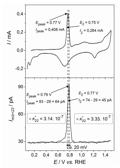
Fig. 11.  $K_{22}^*$  calibration using a CO-stripping CV in 0.5 M H<sub>2</sub>SO<sub>4</sub> on Pt/C and its associated mass-to-charge signal m/z = 22.
