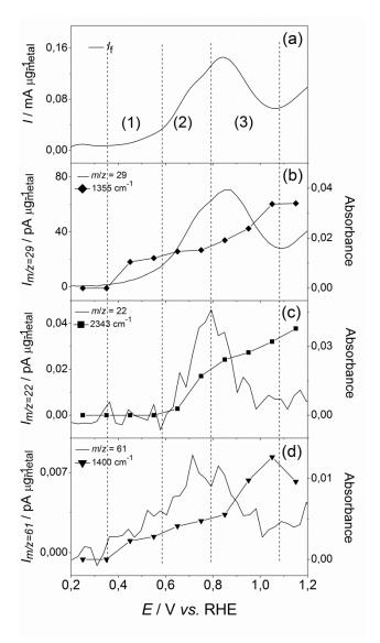
Fig. 33. (a) EOR cyclic voltammetry (in 0.5 M H<sub>2</sub>SO<sub>4</sub> + 0.1 M EtOH) and corresponding MSCV associated with EOR infrared bands (from Fig. 32b): (b) m/z = 29 + 1355 cm<sup>-1</sup>, (c) m/z = 22 + 2343 cm<sup>-1</sup> and (d) m/z = 61 + 1400 cm<sup>-1</sup> on Pt/C; v = 10 mV s<sup>-1</sup>;  $T = 25^{\circ}$ C.
