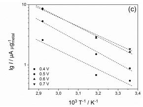
Fig. 81. Arrhenius plots of the of potentiostatic currents recorded after 900 s at potentials from E = 0.4 to 0.7 V vs. RHE (0.1 V step) in 0.5 M H<sub>2</sub>SO<sub>4</sub> + 0.1 M EtOH on (a) Pt/C, (b) Pt-Rh/C and (c) Pt-Rh-SnO<sub>2</sub>/C.
