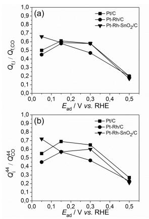
Fig. 73. Relative coverage of Pt/C, Pt-Rh/C and Pt-Rh-SnO<sub>2</sub>/C electroactive surface by acetaldehyde CO-like adsorbates adsorbed at  $E_{ad} = 0.05$ , 0.15, 0.3 and 0.5 V vs.RHE deduced from (a) faraday charges and (b) ionic charges from the mass-to-charge signal m/z = 44.
