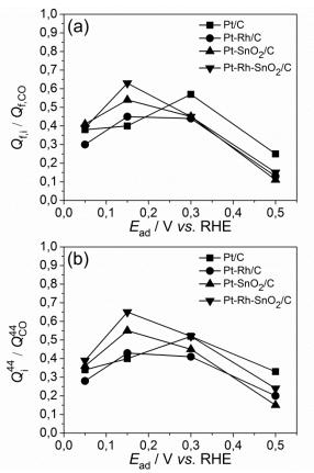
Fig. 70. Relative coverage of Pt/C, Pt-Rh/C, Pt-SnO<sub>2</sub>/C and Pt-Rh-SnO<sub>2</sub>/C electroactive surface by ethanol CO-like adsorbates (oxidizing at 0.4 V < E < 0.9 V vs. RHE) adsorbed at  $E_{ad} = 0.05, 0.15, 0.3$  and 0.5 V vs.RHE deduced from (a) faraday charges and (b) ionic charges from the mass-to-charge signal m/z = 44.
