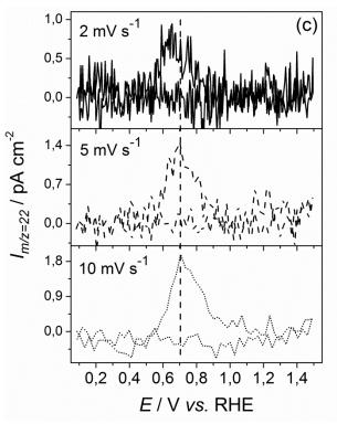
Fig. 22. (a) CV of the EOR in 0.5 M H<sub>2</sub>SO<sub>4</sub> + 0.1 M EtOH on Pt/C and corresponding MSCV for mass-to-charge ratio (b) m/z = 29 and (c) m/z = 22; at v = 2, 5 and 10 mV s<sup>-1</sup>;  $T = 25^{\circ}$ C.
