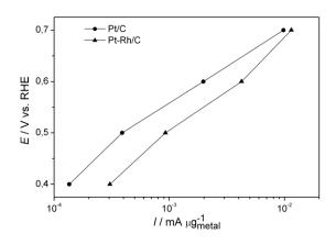
Fig. 86. Tafel plots of potentiostatic EOR currents (after 5 min) on (a) Pt/C and (b) Pt-Rh/C electrocatalysts in  $0.5 \text{ M H}_2\text{SO}_4 + 0.1 \text{ M EtOH}$  at room temperature.
