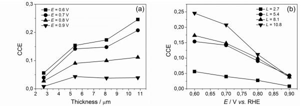
Fig. 16. Evolution of the EOR CO<sub>2</sub> current efficiency (CCE) against (a) the electrocatalyst thickness and (b) the applied potential calculated from cyclic voltammetries run in 0.5 M  $H_2SO_4 + 0.1$  M EtOH (represented in Fig. 15a) and corresponding MSCVs (Fig. 15b) on Pt/C.
