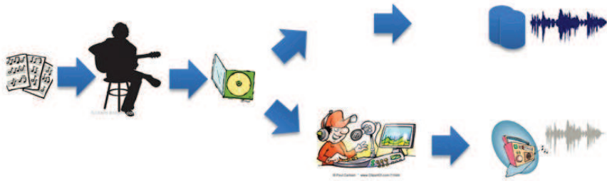
Figure 8.3: Illustration of the exact matching use-case. The algorithm has to match two signals that correspond to the same recording with different post-processing distortions.
