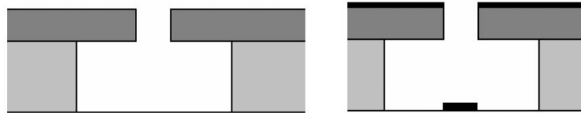
Figure 1.26. Undercut resist profile for clean lift-off [130].
