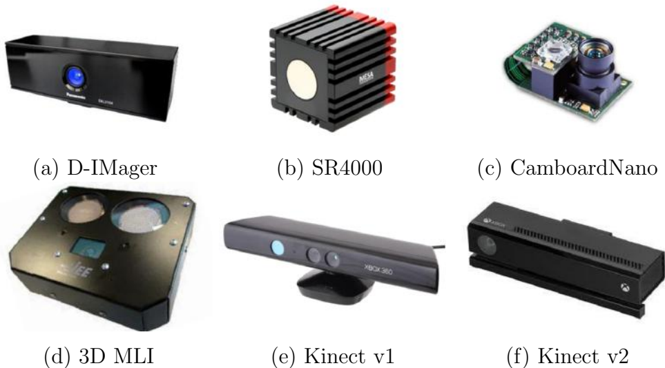
Figure 1.1: Example of depth Cameras. (a) D-IMager by Panasonic – ( 160 \times 120 ) pixels [1], (b) SwissRanger SR4000 ToF camera by MESA Imaging – ( 176 \times 144 ) pixels [2], (c) CamboardNano ToF camera by PMD – ( 160 \times 120 ) pixels [3], (d) 3D MLI Sensor ToF camera by IEE – ( 56 \times 61 ) pixels [4], (e) Kinect v1 structured light camera by PrimeSense – ( 640 \times 480 ) pixels [5], (f) Kinect v2 ToF camera by PrimeSense – ( 640 \times 480 ) pixels [5].
