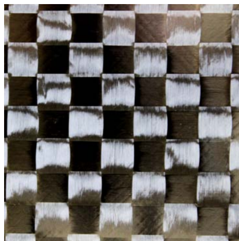
Figure 2.7: Overview of the 12K woven textile preform.
