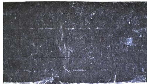
(b) Delamination inside non-crimp fabric specimen for interlaminar shear tests with a angle of 45° according to the fibre direction.
