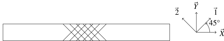
Figure 3.9: Material coordinate system (\vec{1}, \vec{2}) according to the specimen coordinate system (\vec{X}, \vec{Y}) for in-plane shear tests.
