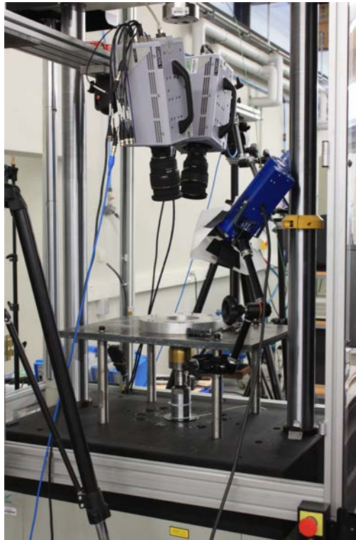
Figure 6.31: Overview of the bulge montage for multi-axial tests on the structure specimen.
