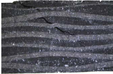
(a) Transverse shear fracture inside 3K woven fabric specimen for interlaminar shear tests in the fibre direction.
