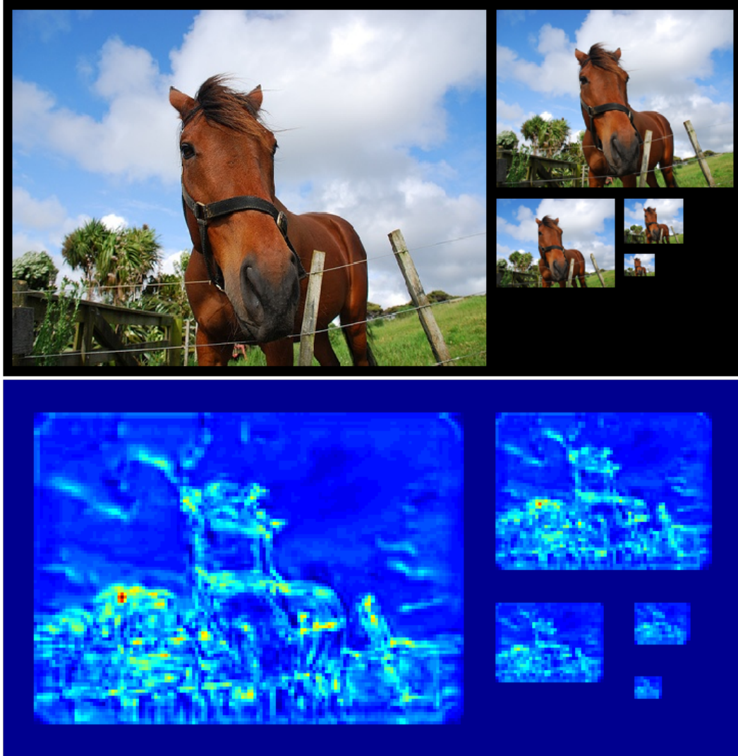
FIGURE 3.14 – Top : We tile rescaled versions of the original image into a single, bigger canvas that can be processed efficiently by the convolutional layers. Bottom : The L^2 norms of the obtained CNN activations in the 5-th layer. After computing convolutions on the patchwork image, we decompose the result into responses corresponding to individual scales and synthesize a pyramid of CNN responses.
