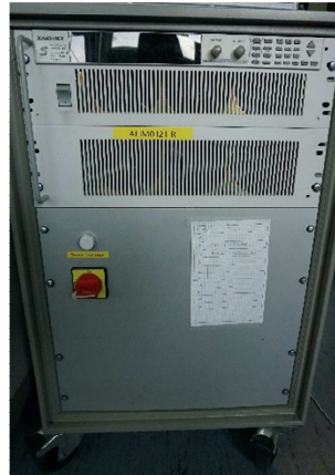
Figure 7.3 Controllable DC source
