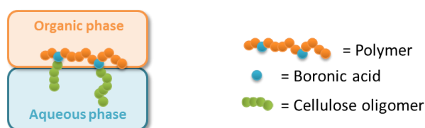
Figure IV-10. Reversible amphiphilic brush copolymer formed at the interface during a “fishing” method with a random copolymer – Scheme not to scale
