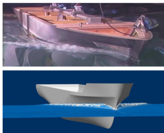
Fig. 21. Breaking bow wave during experiments at DGA-Hydrodynamics (top) and 3D view of the breaking bow wave in the SPH simulation Ship4 (bottom plot), Fn 0.328.
