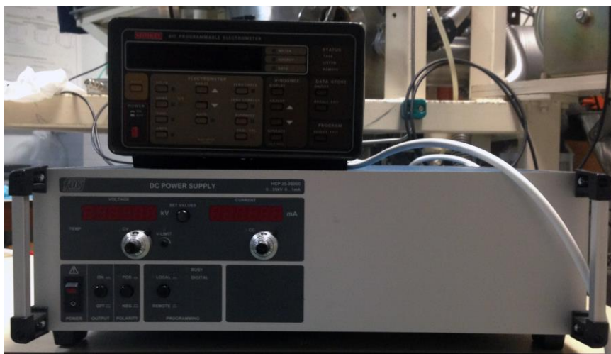
Figure 2-11 Keithley 617 programmable electrometer and DC power supply (voltage up to 35 kV, current up to 1 mA).
