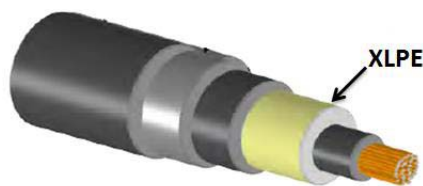
Figure 2-1 XLPE insulation in a power cable.
