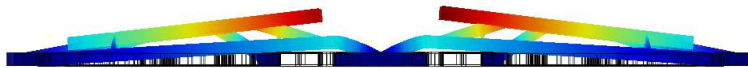
Figure 145: Sense mode (Dynamic acceleration) obtained by FEM for a coupled accelerometer-gyroscope structure (20.0 kHz)
