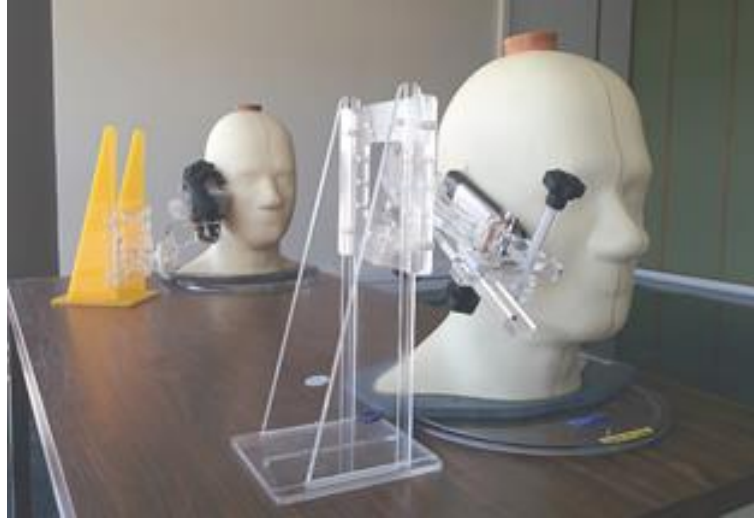
Figure 2.7-i: Setup used for comparing the effect of the hand phantom on the uplink transmit level.
