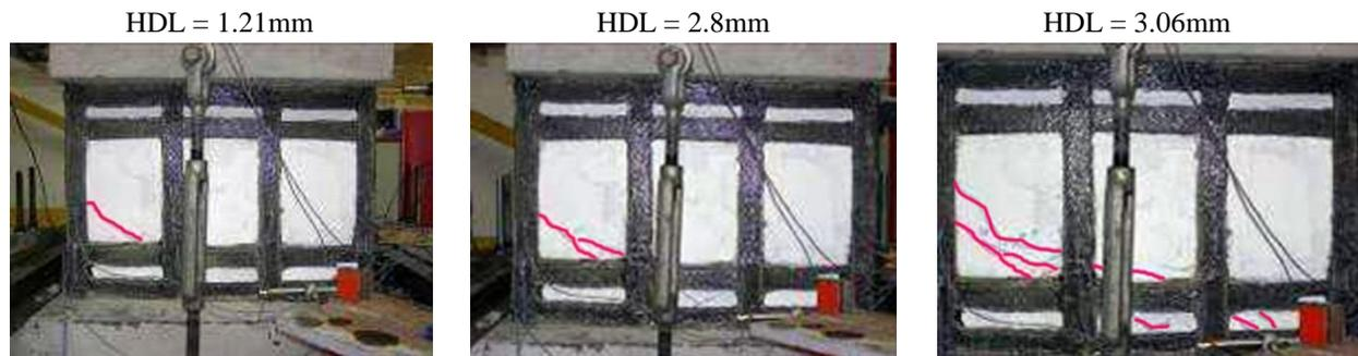
Figure. A-11: Crack pattern of the CFRP-retrofitted short wall VC1
