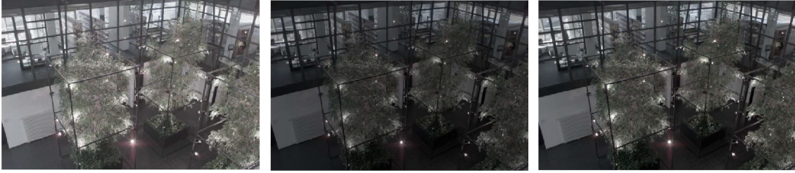
Figure 5.8: Left: TM output using the Michaelis-Menten equation. Middle: TM output using a logarithmic mapping (Weber-Fechner's law). Right: TM output of the first stage of our method, eq. 5.6.
