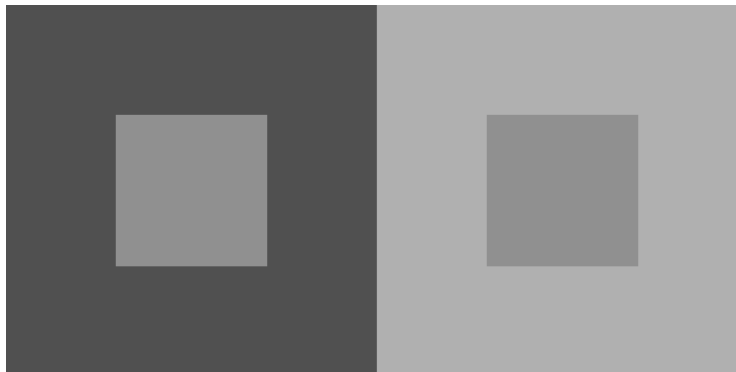
Figure 2.8: Simultaneous contrast: even though the two inner squares have the same luminosity, our perception is different, due to the different background.
