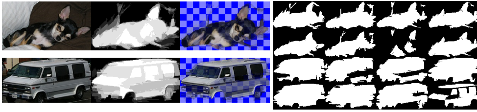
Figure 2.1 – Segmentation masks for two detection windows. The first three columns show the window, our weighted mask, and the masked window. The eight images on the right show the individual binary masks of superpixels lying fully inside the window, for each of eight segmentations.
