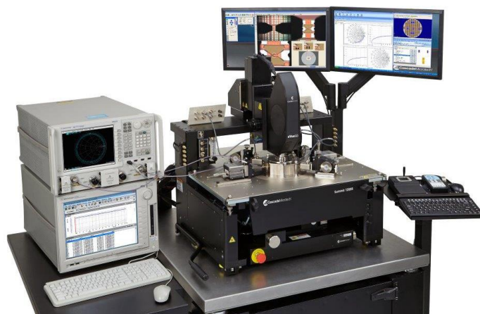
Figure 1.14. On-Wafer Measurement Setup (Cascade Microtech Probe Station)
