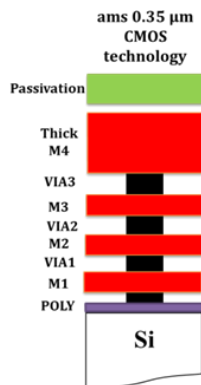
Figure 4.1. Back End of Lines (BEOL) of AMS 0.35 \mu\text{m} CMOS Technology
