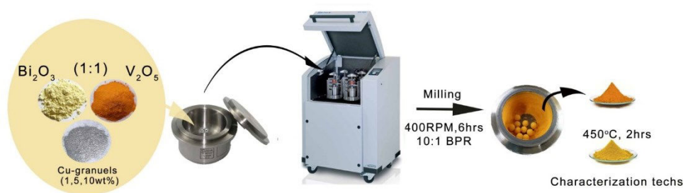
Fig.1.2. Schematic illustration of steps followed in the mechano-chemical synthesis of doped \text{BiVO}_4 nanoparticles with several dopants.
