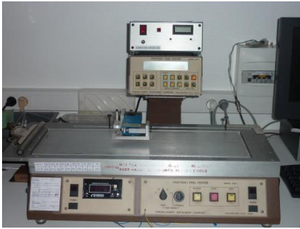
Figure 2.13. a) Picture of peel tester. b) Schematic of the peel test for a linearly elastic, extensible adhesive tape [119]
