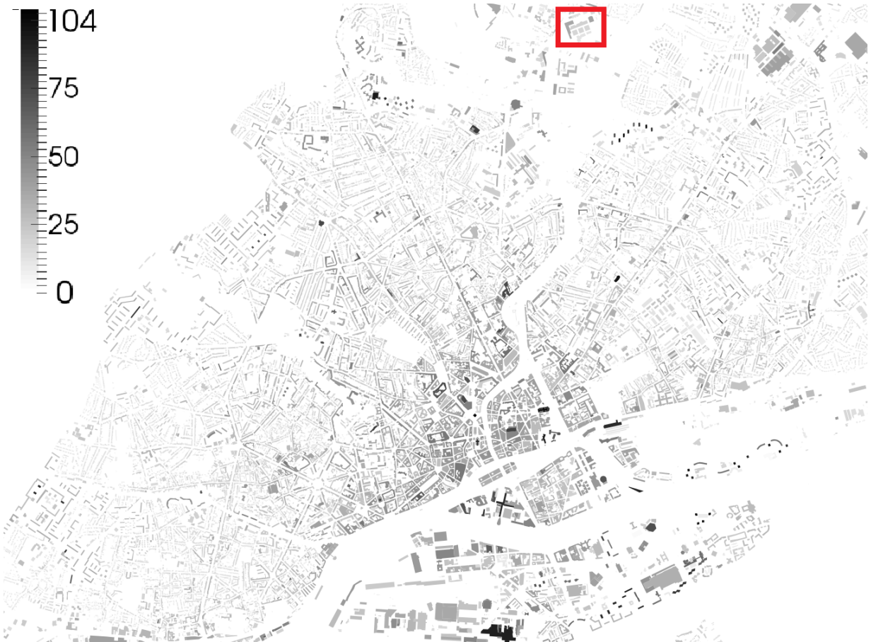
Figure 4.19: 2D image representing the urban (building) description of Nantes, obtained using the GIS 's database of BDTopo , through IRSTV.
