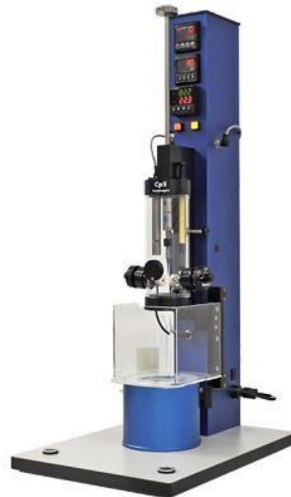
Cryoplunge™3 for the preparation of frozen hydrated specimens for cryo-EM Gatan.com
