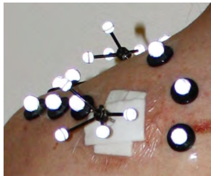
Figure 78 : Intracortical pins and tape positioning near the scapula for Jackson et al. marker set
